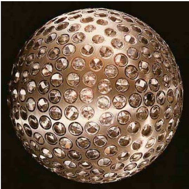
Figure 11. The LAGEOS-1 satellite (identical to LAGEOS-2). Dedicated laser ranging satellites have a long-term orbital stability because of their spherical shape and high mass-to-area ratio.
