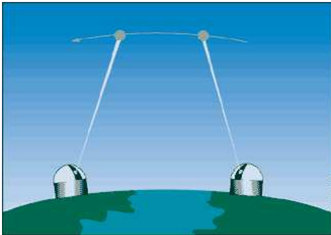
Figure 10. Principle of satellite laser ranging.
